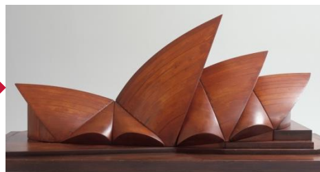
Arup wind tunnel model
